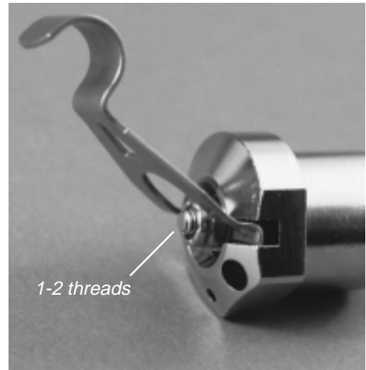
Fig. 12 – Locknut Preliminary Setting
