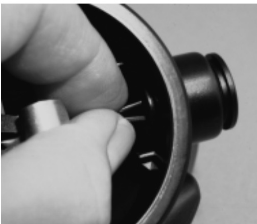
Fig. 2 – Removal of End Plug
