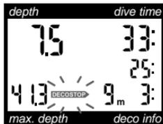
**Messages:** The decompression alarm is activated if the decompression stop is ignored. Arrow <DECOSTOP> flashes and an acoustic alarm is initiated. Due to the formation of microbubbles decompression can increase massively while a decompression stop is ignored. If the surface is reached during the decompression alarm, the arrow <DECOSTOP> continues flashing, in order to point to the risk of a decompression accident. The SOS-mode is activated after 3 minutes after the dive.
