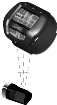
1. Each transmitter works with an allocated address. This address is communicated to the dive computer on pairing. There are more than 60,000 addresses. This assures that no two transmitters send on the same channel. The pairing of transmitter and receiver is also carried out by a process with various safety levels in order to prevent faulty pairing.
