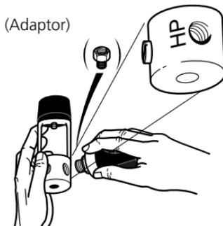
Fit the transmitter to the HP outlet. If the threads do not match, get an adaptor from your diving retailer.
