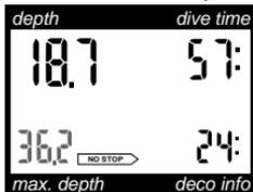
The maximum depth is only displayed if it exceeds the current depth by more than one metre. This is to prevent the display changing very frequently when diving in the vicinity of the maximum depth.
