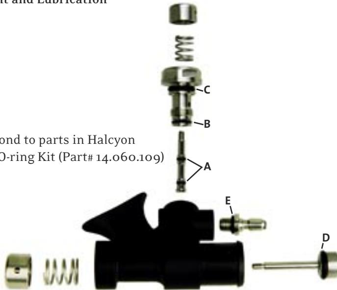
All O-rings should be replaced during servicing. The appropriate O-rings are marked to match the Halcyon Power Inflator Repair Kit. O-rings can be removed using an O-ring pick. Be sure not to damage the O-ring during installation. All O-rings need to be lubricated with a NSF-61 approved silicone compound lubricant.
